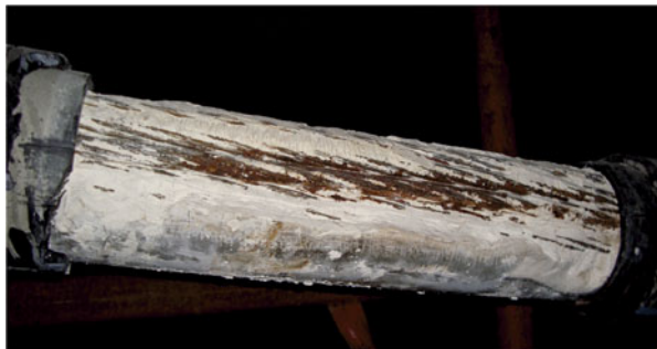
Figure 5. Example of an aperture in the duct of a tendon showing the whitish segregated grout embedding corroding strands.
