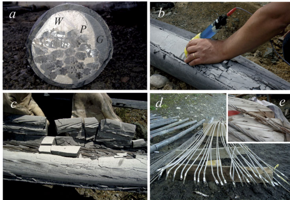
Figure 8. Inspection of a tendon removed from the bridge: (a) types of grout observed on a cutting section, (b) measurement of the corrosion potential of steel strands, (c) inspection of the grout, (d) inspection of the steel strands and (e) detail of wires of a strand broken due to corrosion.
